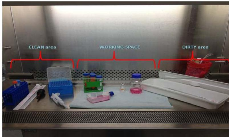
Figure 2: Proper setup when working in a BSC.
