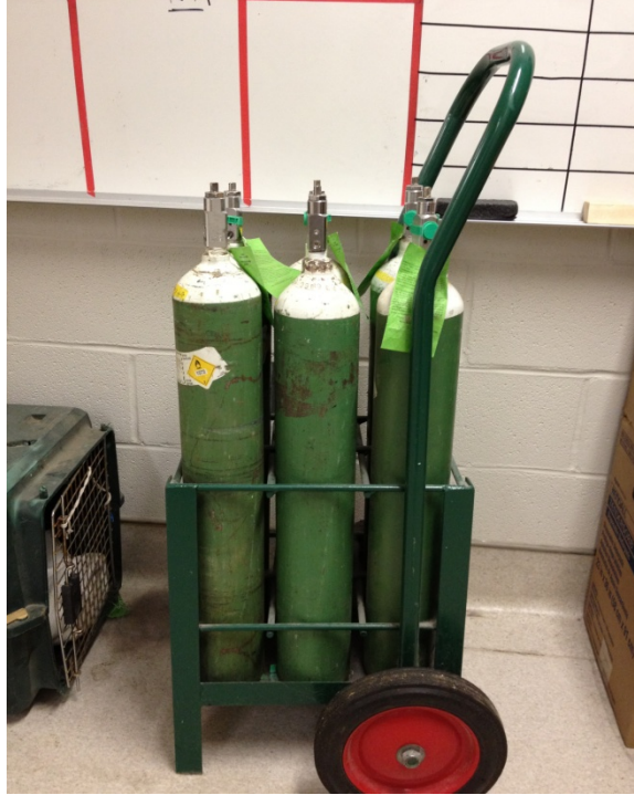
Figure 7: Example of a cylinder cart. Image courtesy of Safety Resources.
