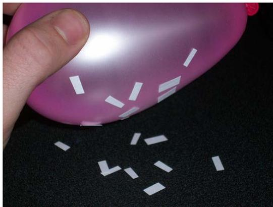
Figure 3: Example of static electricity. Pieces of paper are shown clinging to a balloon as a result of a buildup of static charge. Image courtesy of njorthr, Flickr.
