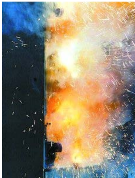
Figure 2: Example of an arc flash. Image courtesy of Plant Engineering.
